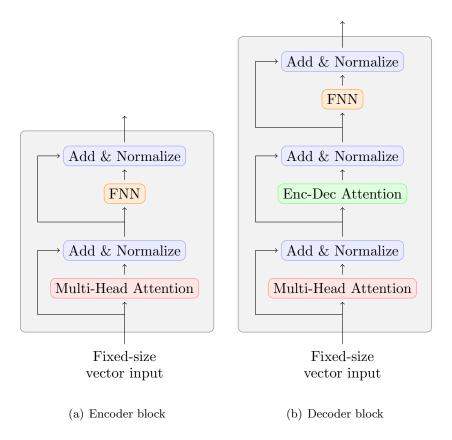
Figure 2: A more detailed architecture of the transformer including separate blocks for the Encoder and Decoder.
